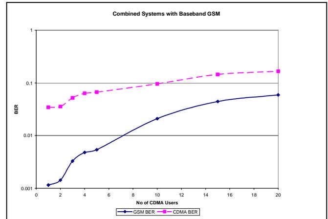
Figure 10: The BER of the Base-band Model
