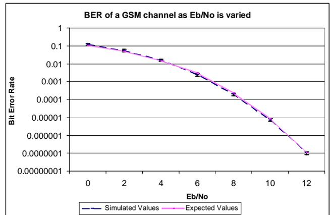
Figure 7: The GSM Calibration Curve (BER of the System as AWGN was Varied)
