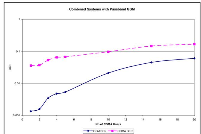
Figure 11: The BER of the Pass-band Model
