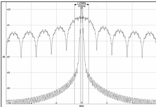
Figure 6: The Spectral Densities of the Separate Systems on one axis
