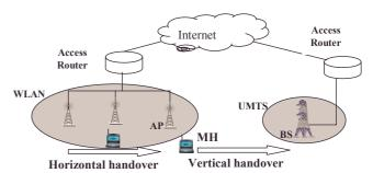
Figure 1: Horizontal and Vertical handover
