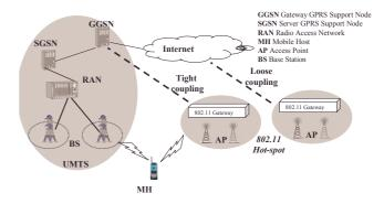
Figure 2: Integrated UMTS/WLAN systems
