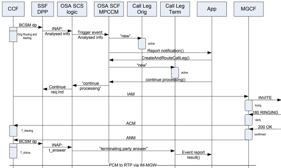
Fig. 7. Circuit Switched Originated Call to IMS subscriber
