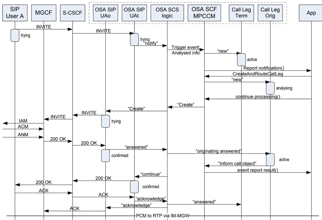
Fig. 8. IMS Originated Call to Circuit Switched subscriber
