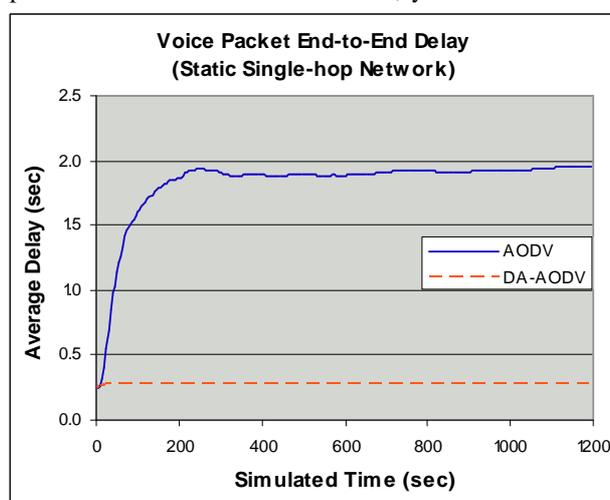
Fig. 2. Static Single-hop Network – Voice Packet End-to-End Delay
