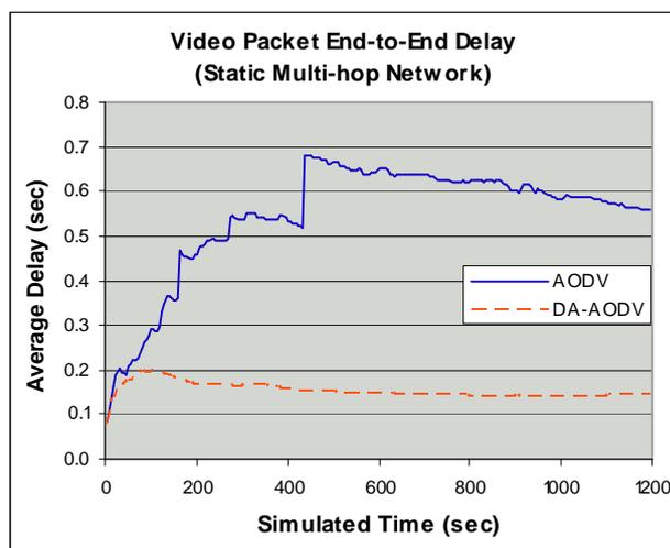
Fig. 3. Static Multi-hop Network – Video Packet End-to-End Delay
