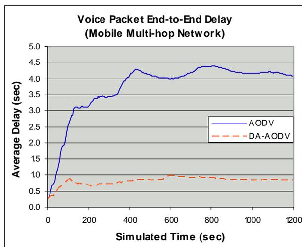
Fig. 8. Mobile Multi-hop Network – Voice Packet End-to-End Delay
