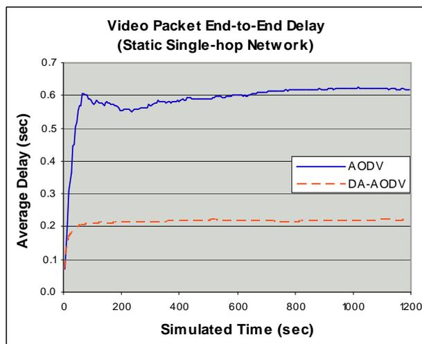
Fig. 1. Static Single-hop Network – Video Packet End-to-End Delay
