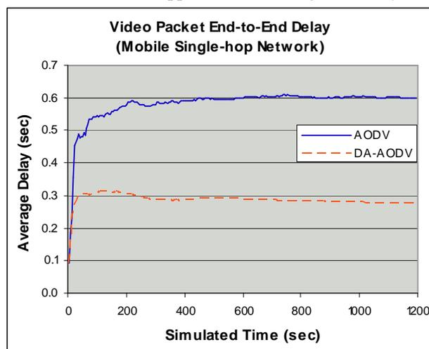
Fig. 5. Mobile Single-hop Network – Video Packet End-to-End Delay
