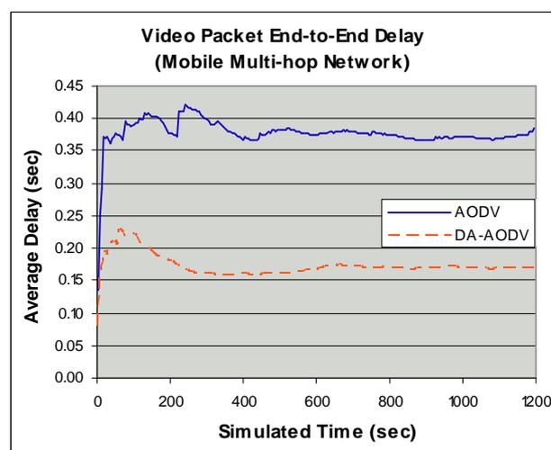
Fig. 7. Mobile Multi-hop Network – Video Packet End-to-End Delay
