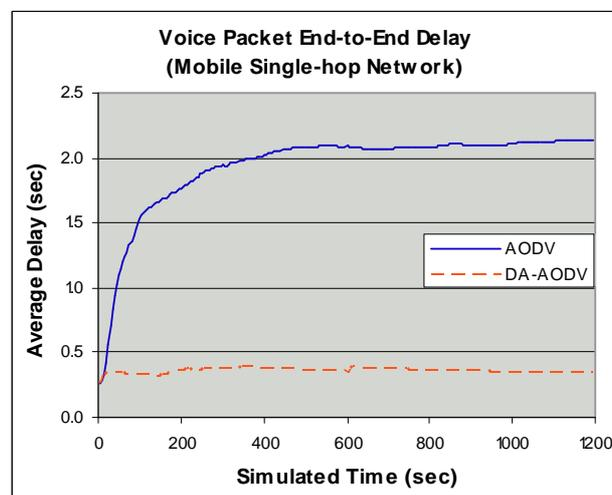
Fig. 6. Mobile Single-hop Network – Voice Packet End-to-End Delay
