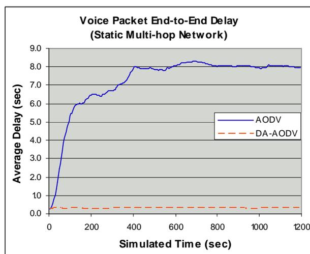
Fig. 4. Static Multi-hop Network – Voice Packet End-to-End Delay
