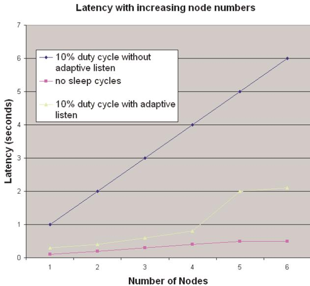
Figure 6. Latency in a linear aligned sensor network
