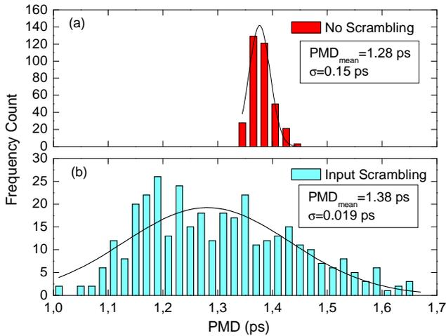
Fig. 6 Gaussian distribution for PMD reading on undeployed aerial optical fibre cable with (a) no polarization scrambling and (b) with input polarization scrambling.
