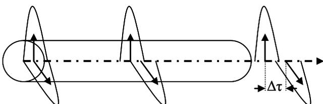
Fig. 1. Schematic illustration of the broadening of the optical pulse through an optical fibre resulting in differential group delay ( $\Delta\tau$ ) [2].
