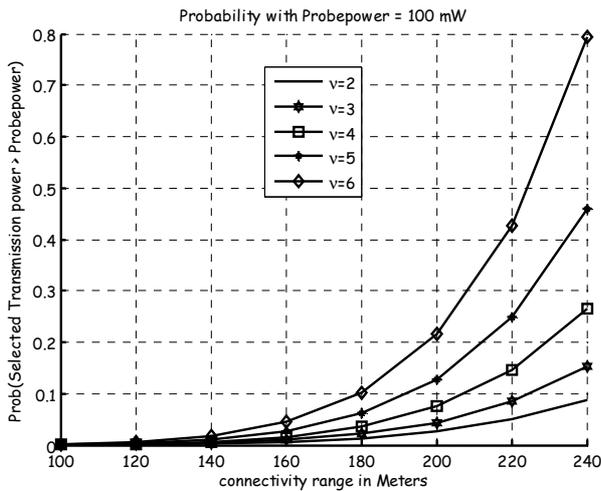
Fig. 4: Transmission Power Probability function versus Range
