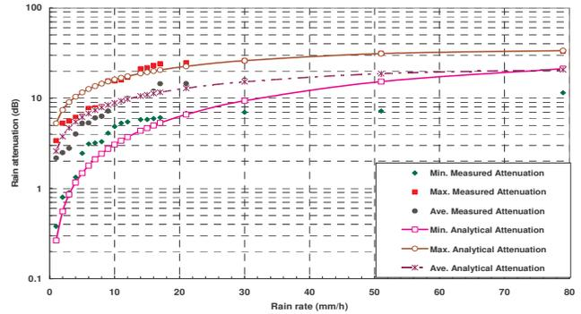
Fig. 4 Best fit analytical rain attenuation for the maximum, average and minimum experimental attenuation values
