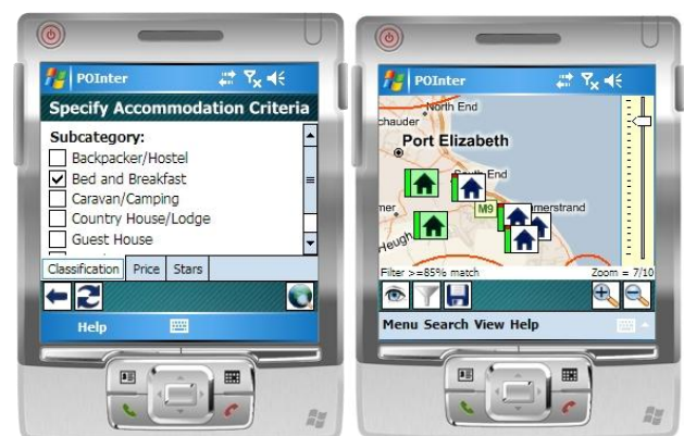
Fig. 1. Specifying criteria (left) and viewing search results using a map (right) in POInter [9].
