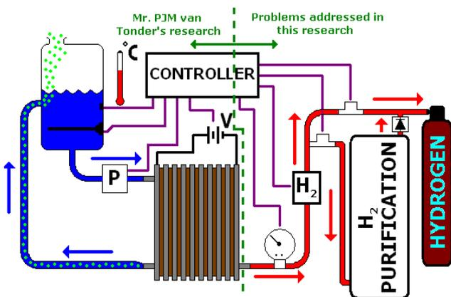
Figure 2 Hydrogen production and control system
