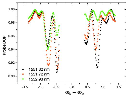
Fig. 2. Variation of probe DOP over the pump spectrum for the probe at 1551.32 nm, 1551.72 nm and 1552.93 nm
