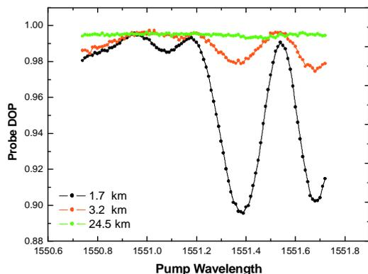
Fig. 3. Probe DOP degradation for fibre lengths 1.7 km, 3.2 km and 24.5 km
