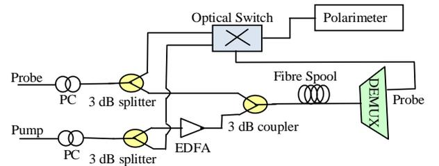
Fig. 1. Experimental setup: A two-channel WDM system (PC = polarization controller)
