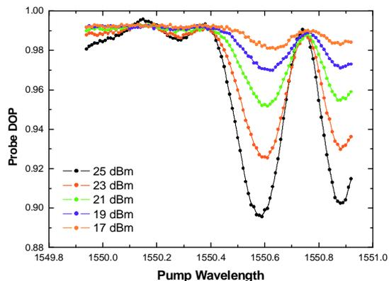
Fig. 4. Effect of varying the input pump power (through EDFA gain)
