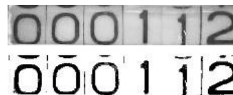
Fig. 1. Meter dials before and after thresholding
