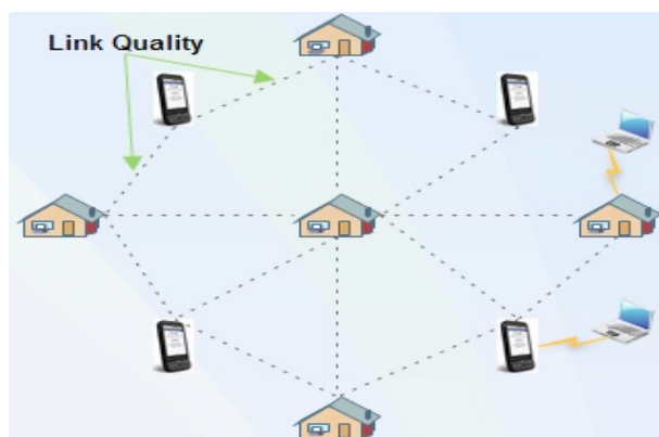
Fig. 1: A hybrid mesh network, applicable to a rural area, with static mesh routers inside homes, and mobile mesh nodes on cell phones. Note that link quality in such networks is continually changing as phones move around.
