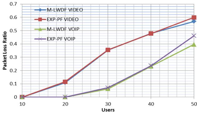
Figure 4 Packet Loss Ratio of Video and VoIP users
