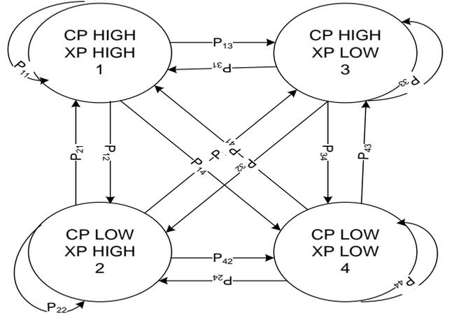
Figure 2 Four-state Markov model of an LMS-MIMO channel
