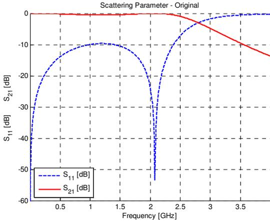
**Fig. 5. Third order Chebyshev low pass filter with a 0.5 dB ripple and cut-off frequency of 2.4 GHz.**
