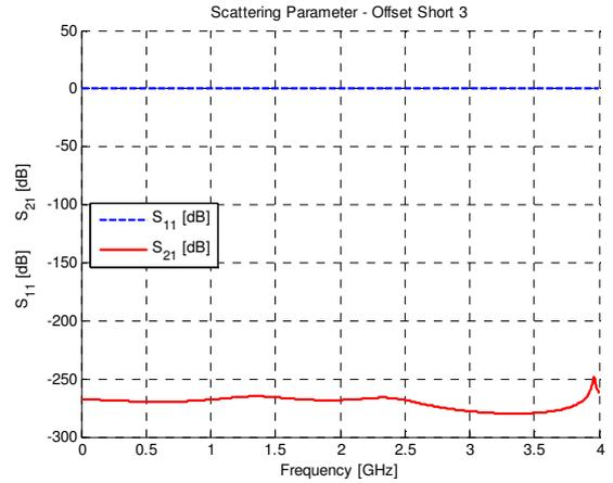
**Fig. 8. Calculated reflection coefficient with third short termination of  $0.50 \lambda$ .**
