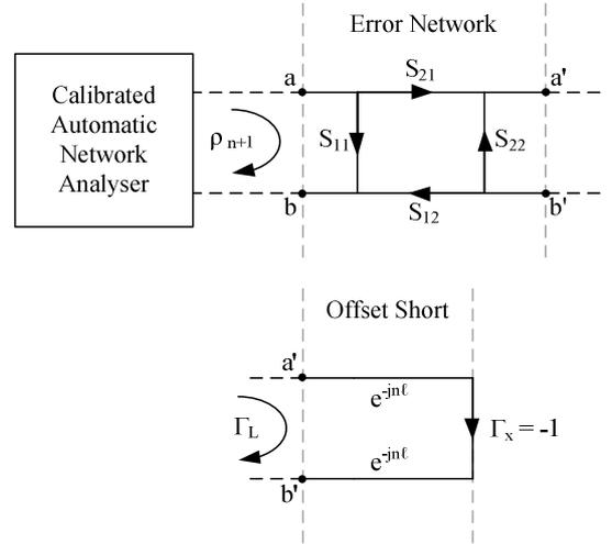
Fig. 4. Graphical representation of the three different offset short configuration for de-embedding. Adapted from [19].
