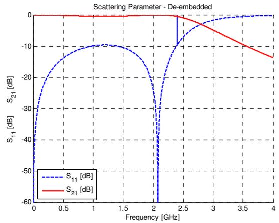
**Fig. 9. De-embedded response of the initial third order Chebyshev low pass filter.**
