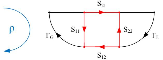
Fig. 1. Signal flow diagram to describe a section of microwave circuit.
