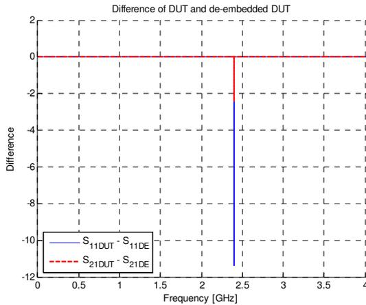
**Fig. 10. Calculated difference between initial and de-embedded network.**
