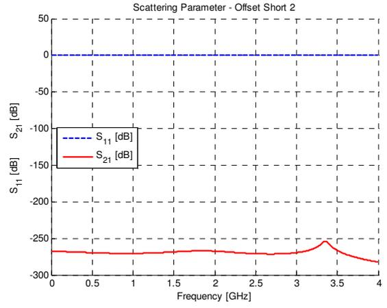
**Fig. 7. Calculated reflection coefficient with second short termination of  $0.25 \lambda$ .**
