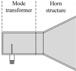
Fig. 2. Mode transformer with a horn structure attached as the load.
