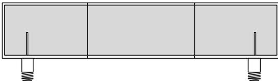
Fig. 3. Back-to-back configuration of two mode transformers with a phase delay between them.
