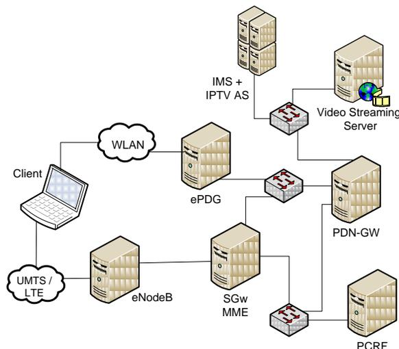
Figure 5: Testbed layout
