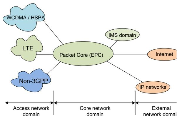
Figure 1: Mobile access and core domains
