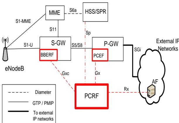
Figure 3: Policy and Charging Control architecture of the EPC.
