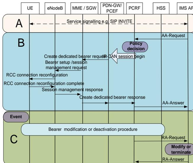
Figure 4: AF signalling procedures with the PCC
