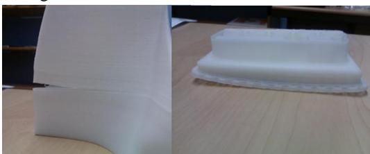
Figure 3 Bow warping effect visible on printed parts
