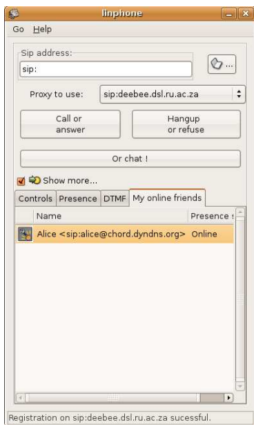
Fig. 6. Presence status of a peer-to-peer user agent displayed on a client-server user agent.
