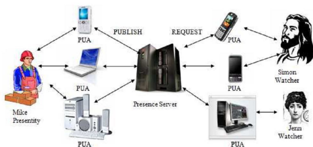
Fig. 2 Sip Presence Architecture
