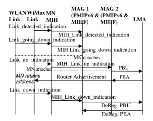
Fig. 5. PMIPv6 enhanced with MIH handover operation.
