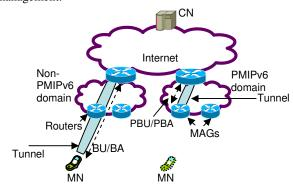
Fig. 1. Illustration of mobility-related signaling flow routes in PMIPv6 and non-PMIPv6 domains.
