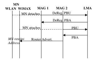
Fig. 4. PMIPv6 handover operation.
