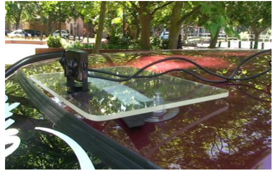
Fig. 3. The specially designed framework on which the cameras rest.
